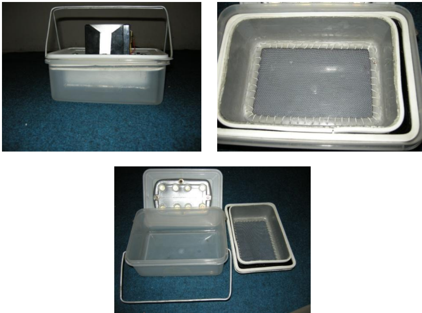
Figure 1. Designing and manufacturing portable and rechargeable separator of terrestrial Arthropods of the soil.
