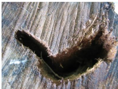
Figure 4. The damage of larvae in the wood.
