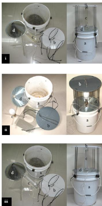
Fig. 5. Disassembled and assembled light traps; UV (i), Mercury (ii) and Black (iii); Collecting chamber (a), Lid from the top (b), Light source (c), Funnel shaped lid (d)
