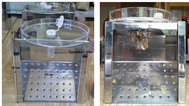
Figure 1. Cages used in the experiments, left: dimensions of the cages, and right: caged bees.
